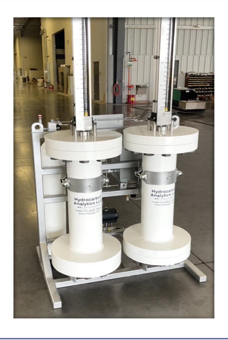
Hydrocarbon Analytics sampling systems are designed to sample light liquid hydrocarbons including NGLs, LPGs, condensates, as well as hazardous chemicals.
